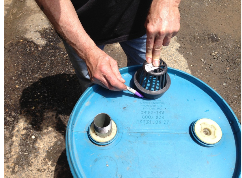
Marking the screen so we can cut the whole for screen
