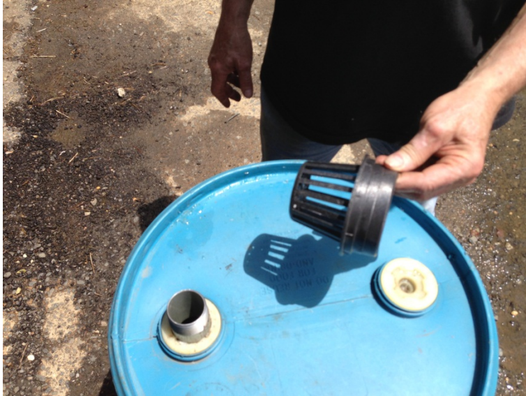
Internal debris screen
