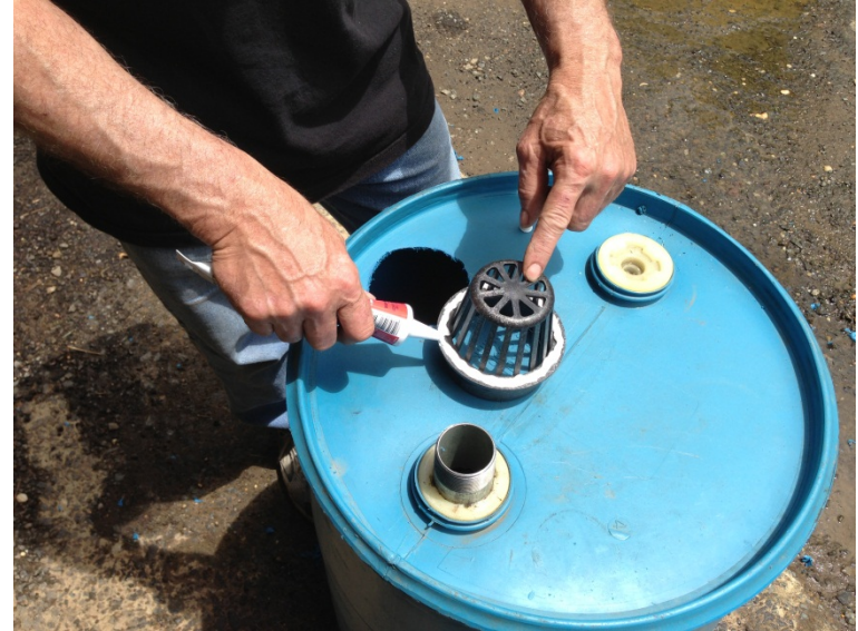
Seal with either screws or silicone
